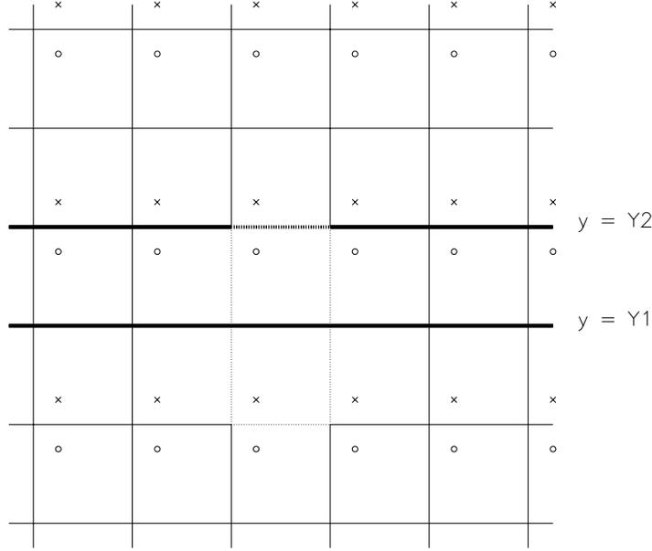
Figure 1.2: Periodic wire array between grounded parallel planes
